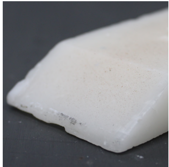
(b) Surface roughness and defects due to manual casting.
