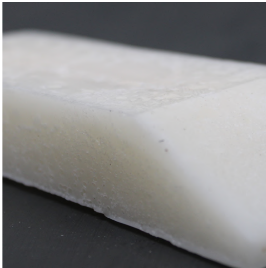
(a) Visible air bubbles on paraffin fuel surface.
