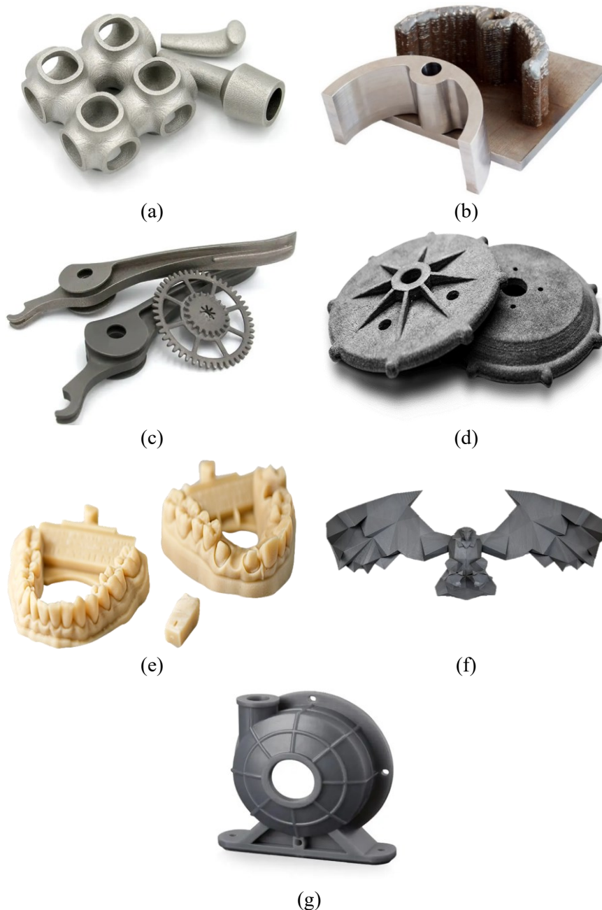
Figura 13 Peças fabricadas por: (a) BJ (SCULPTEO, 2022), (b) DED (FITNIK, 2022), (c) PBF (SCULPTEO, 2022), (d) SL, créditos da Impossible Objects (ENGINEERING PRODUCT DESIGN, 2022), (e) MJ (3D SYSTEMS, 2017), (f) ME (SCULPTEO, 2022) e (g) VP (FORMLABS, 2020).
