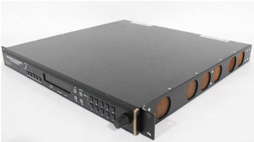
Figura 18 – Master Clock/SPG model 5600MG [25].
