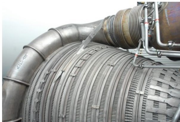
Figura 6 – F1 engine cooling pipes running through nozzle structure (WIBERG, 2019)
