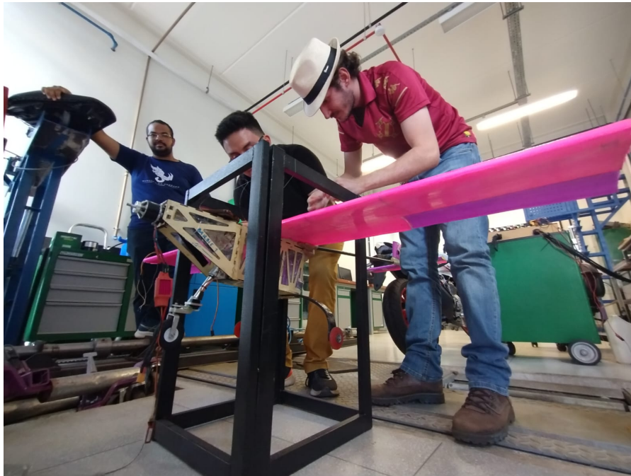
Figure 4.13: Barbie suspended in the air by nylon cables. To avoid frontal movement of the plane, the propeller was removed from the plane's motor.
