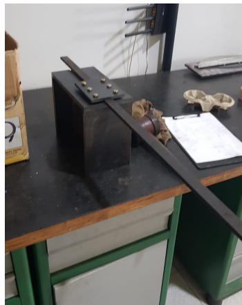
(b) The beam and secondary plates are fixed in position with six screws attached to self-locking screws.
