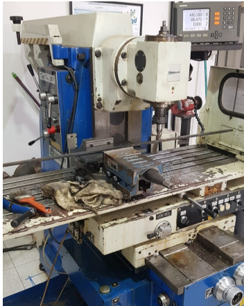
(a) Milling machine used to create the central channel on the main plate.
