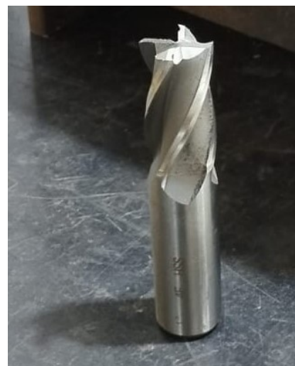
(b) CNC End mill used to create the central channel of the main plate
