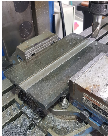
(b) Central channel created with the milling machine.
