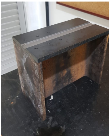
(a) The main plate was welded with the I-beam. The combined weight of this components serve their positions with six screws attached to self-locking screws.
