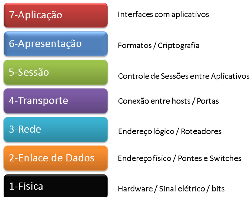
Figura 1 – Modelo OSI (Open Systems Interconnection)
