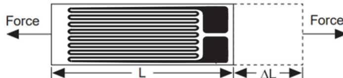
Figure 9 – Strain Gauge adapted from (INSTRUMENTS, 1998).
