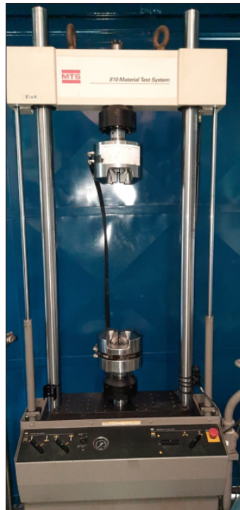
Figura 12 – MTS 810 Material System, Brasília - UnB,SG9.
