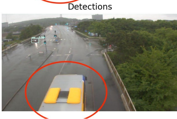
(a) False negative due to out-of-frame object
