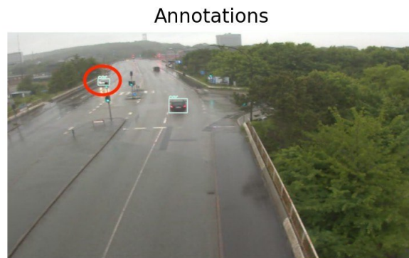
(b) False negative due to distance and object size.
