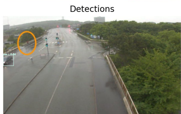
(b) False negative due to distance and object size.
