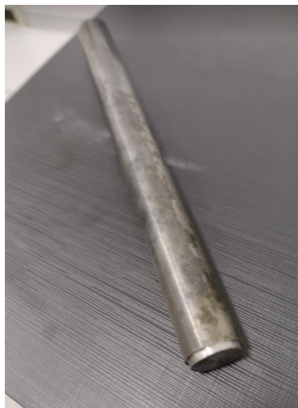
Figure 52 – 217 mm bar after lathe machining with lower size dimensions in its borders.
