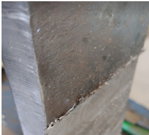
Figure 47 – Lower plate after machining process, presents burrs.
