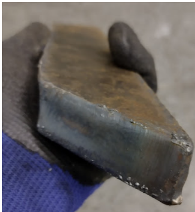
Figure 39 – Trapezoidal support with iron oxide and burrs.
