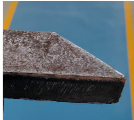
Figure 40 – Trapezoidal support with iron oxide but without burrs.
