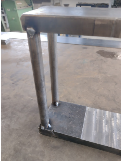
Figure 57 – MIG weld point applied between the plates and the bars.
