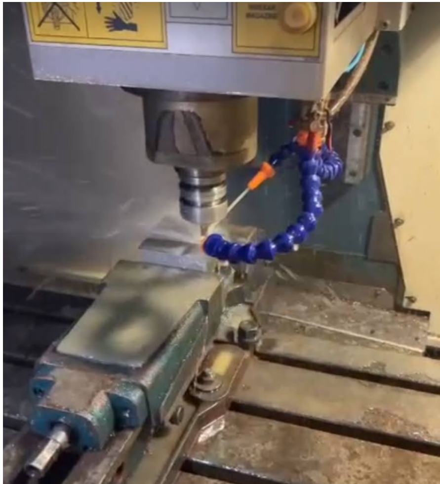
Figure 53 – CNC Milling Process to machine the mould.
