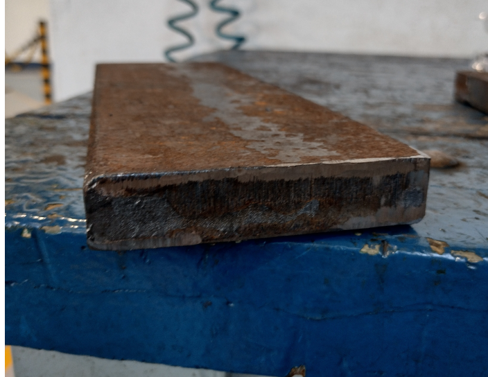
Figure 38 – Plate with iron oxide but without burrs.
