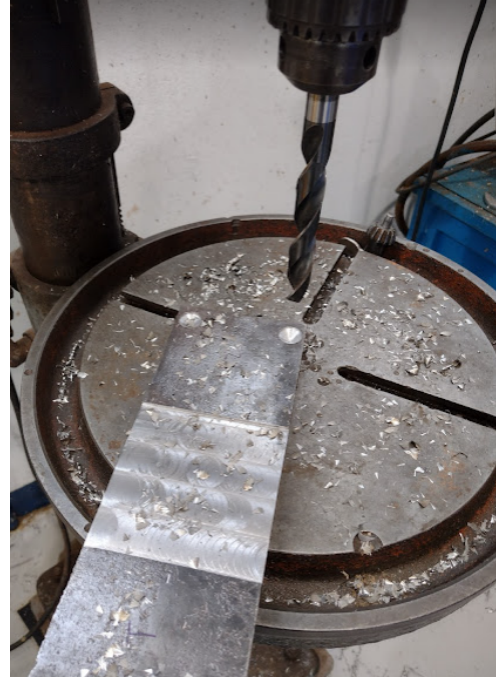
Figure 46 – Inferior plate after the 17 mm diameter holes drilled.
