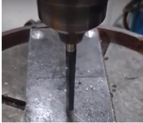
Figure 49 – Drilling superior’s plate middle hole.
