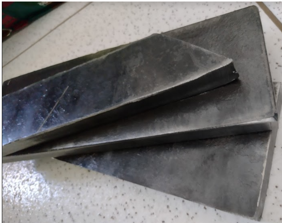
Figure 43 – Support and Plates without burrs and iron oxide.
