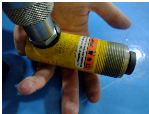
Figure 5 – Photo showing the Enerpac's RC-51 actuator used in this project.
