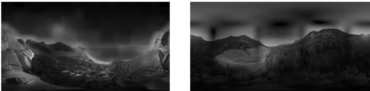
Figure 4.3: Examples of saliency maps generated by the two algorithms analysed, Cube Padding and BMS360. The image on the left shows the BMS360 saliency and the image on the right shows the Cube Padding saliency map. We can easily see the borders of the cube in this projection.
