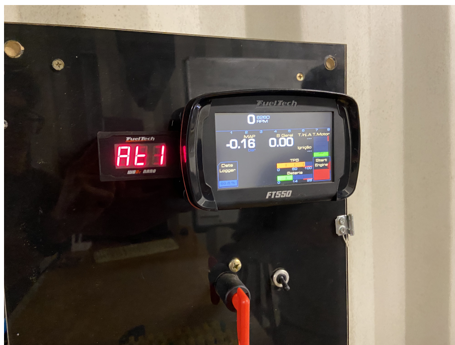
Figura 10 – Painel da ECU FuelTech FT550
