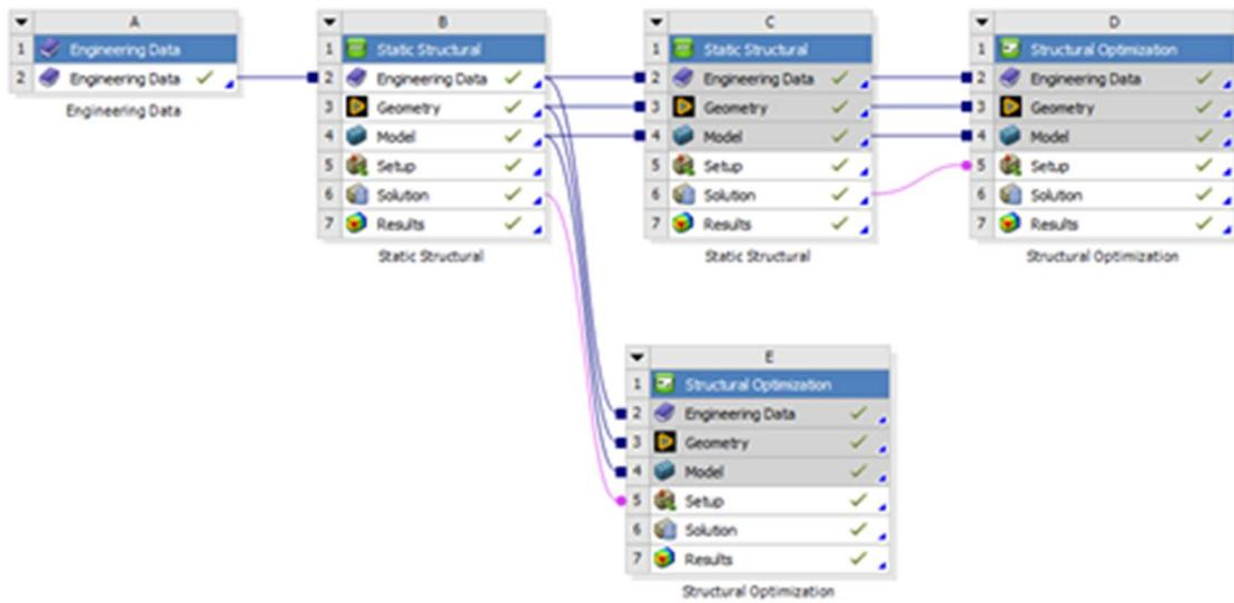
Figure 6. Example of topology optimization Workbench tree.
