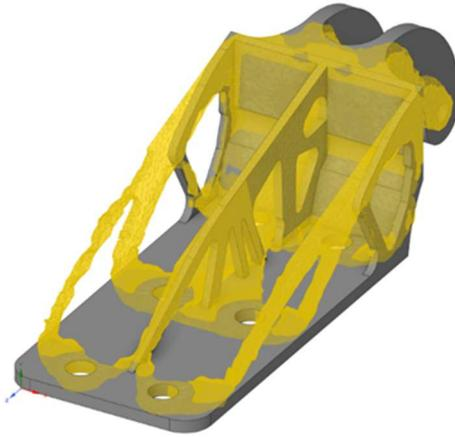
Figure 28. Comparison between optimization results from load case 1 and the final obtained geometry.
