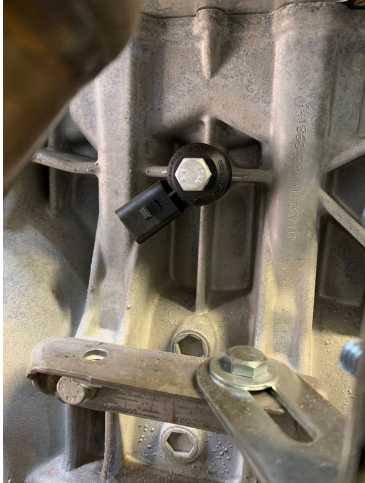
Figura 54 – Sensor Knock do motor EA211
