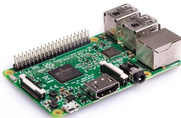
Figura 5 – *Raspberry pi 3 model b*
