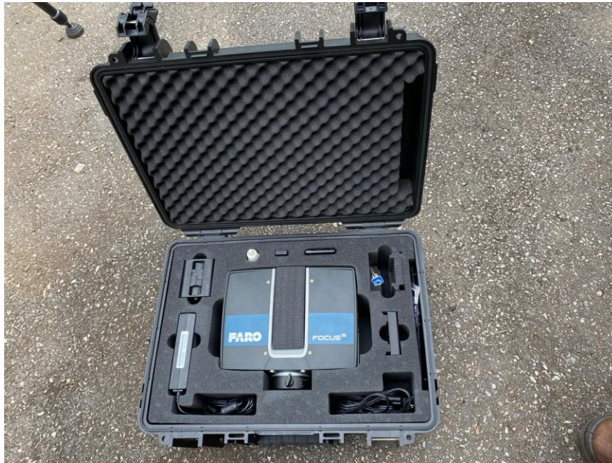
Figura 5-7: Laser Scanner FARO Focus M 70
