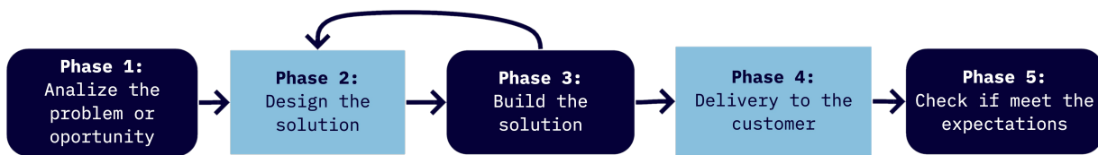
Figura 1 – The five phases of the product engineering workflow. The development consists of a cycle that allows feedback loops at any stage. In Phase 3, the presented feedback loop arrow aims to ensure greater alignment between the Build and Design the Solution.
