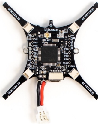
Figure 15 – Bottom of the Crazyflie main board, that also is the main structural component of the drone.
