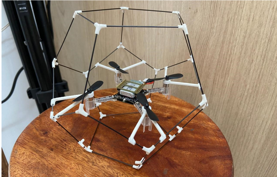
Figure 10 - Complete assembly of the dodecahedron structure with the drone docked.
