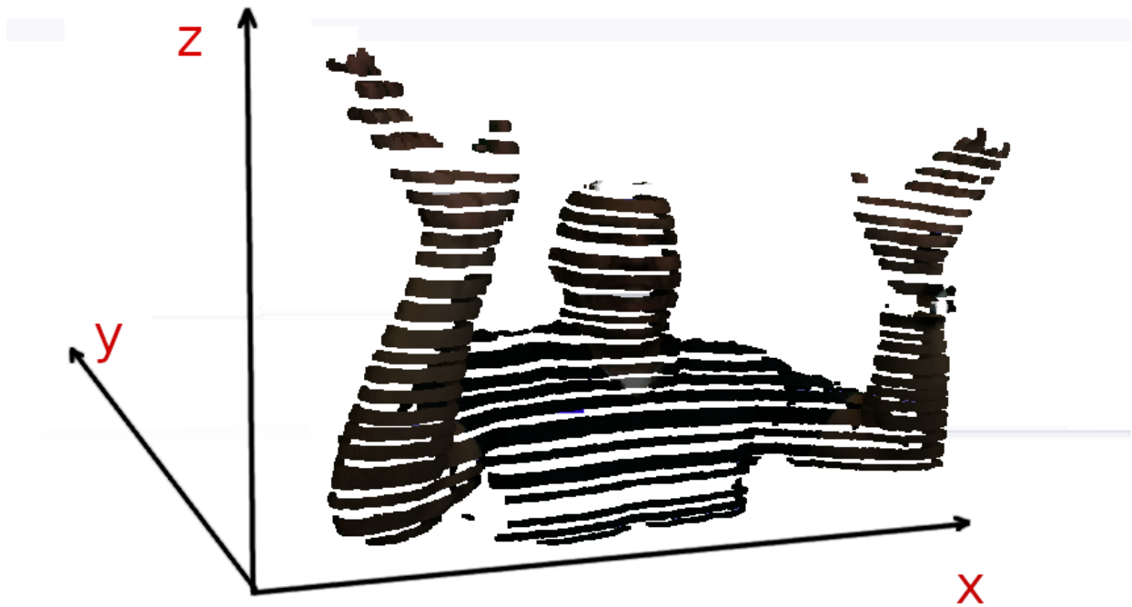
Figure 2.10: An illustrative purpose image depicting slices images from decode - leaf nodes - merged and reconstituting the original point cloud on axis Y.
