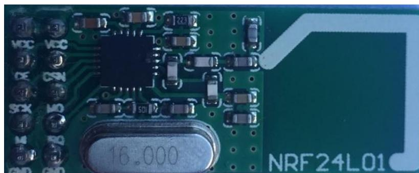
*Figura 3.10. Radio digital nRF24L01*
