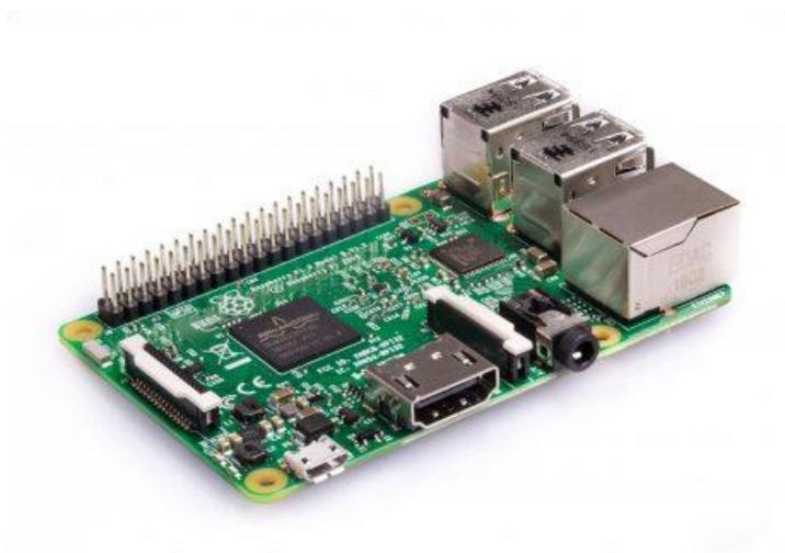
Figura 2. 1- *Raspberry Pi 3 Model B* [5].
