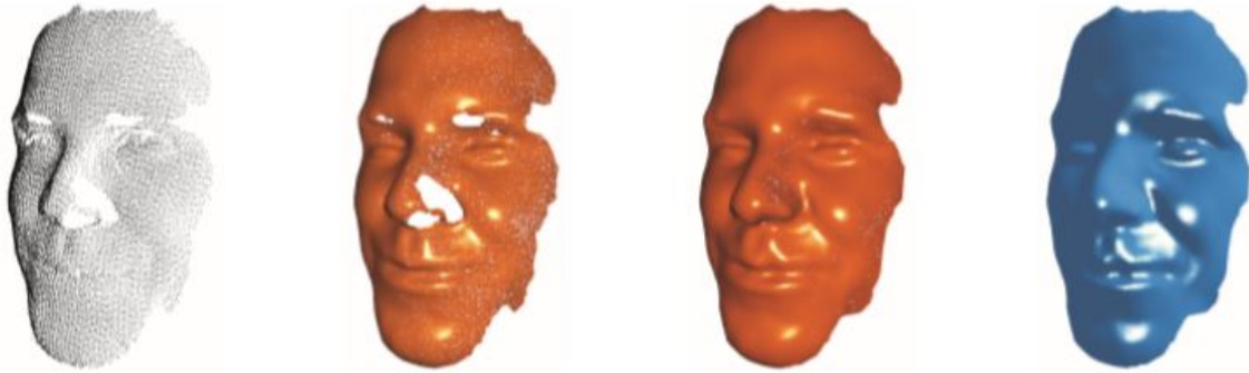
Figure 2.5 – Scanned Data, Reconstruction, Manual Hole Filling, Final Rendering[3]
