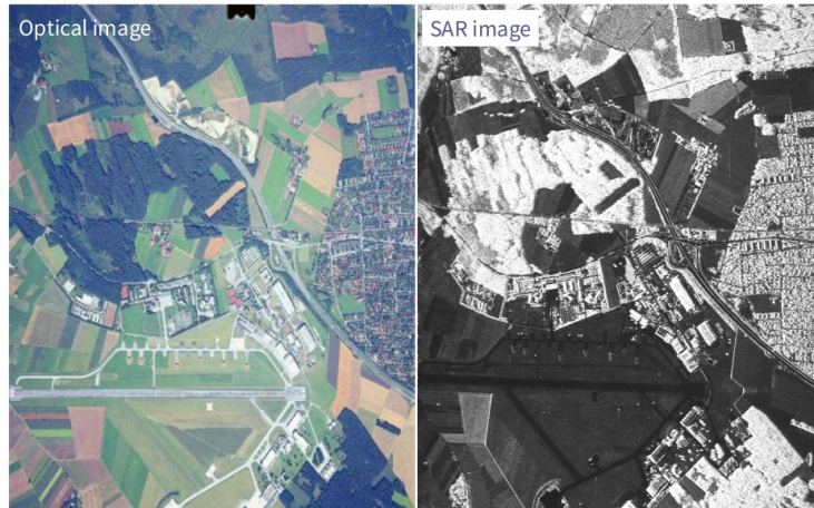
Figure 1.1: Optical and SAR images of the same scene. We can see that the interpretation of the image is a bit more nuanced in the SAR case than in the optical case, since SAR obtains the reflectivity of the scene, instead of properties like color. Image taken from [23].
