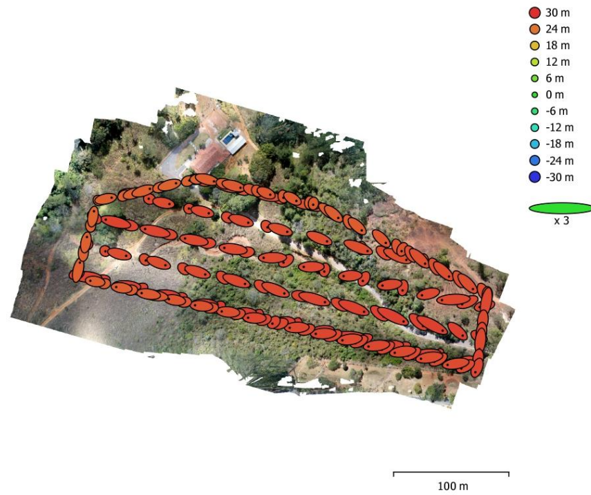
Fig. 3. Camera locations and error estimates. Z error is represented by ellipse color. X,Y errors are represented by ellipse shape. Estimated camera locations are marked with a black dot.
