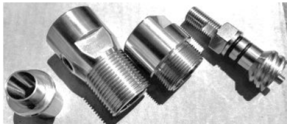
Figura 10 – Componentes do ignitor (SOUZA; SHYNKARENKO, )
