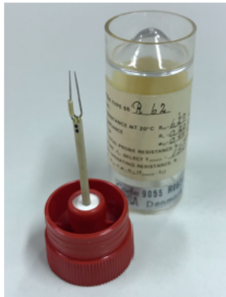
Figura 16 – Sonda Unidimensional DISA 55R 62 (CINTRA, 2017).
