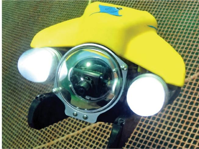
Figura 2.2: ROV VideoRay 4 Pro
