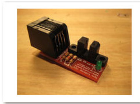
Figura 5.4: Opto Endstop v2.1
