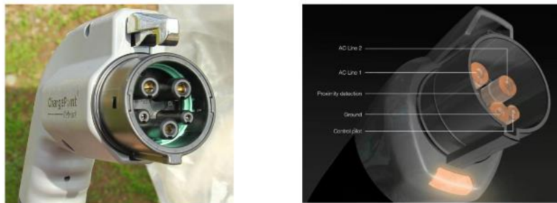
Figura 19. Conector SAE J1772
