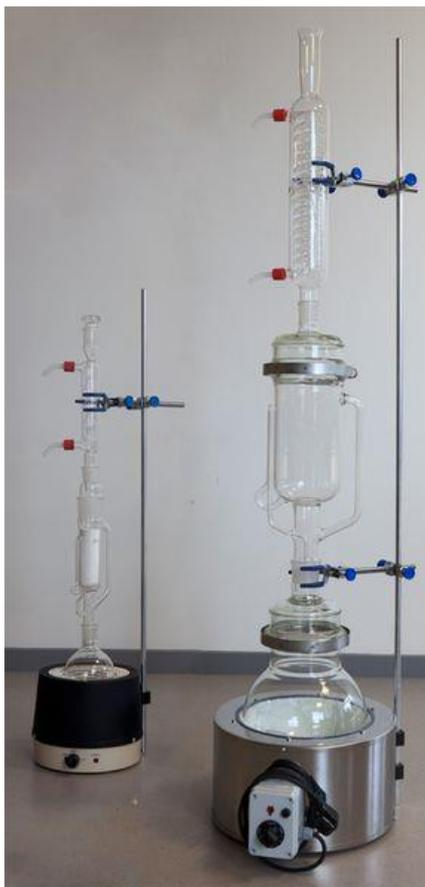
Figura 11. Extrator de Soxhlet. Fonte: <http://www.vinci-technologies.com/products-explo.aspx?IDR=82293&idr2=82573&idp=82288&IDM=536742>
