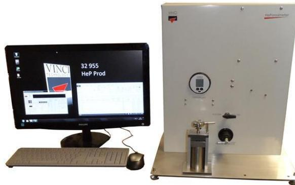
Figura 15. Porosímetro de hélio. Fonte: <http://www.vinci-technologies.com/products-explo.aspx?IDR=82292&idr2=82524&idp=82288&IDM=536752>
