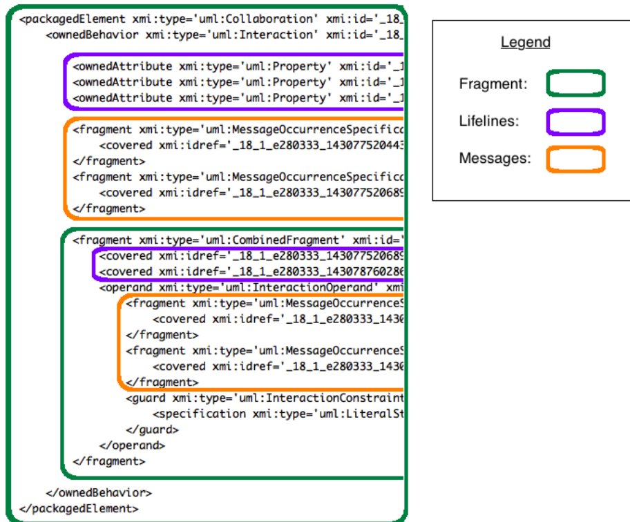
Figure 4.4: Fragment of an XML Representation of a Sequence Diagram
