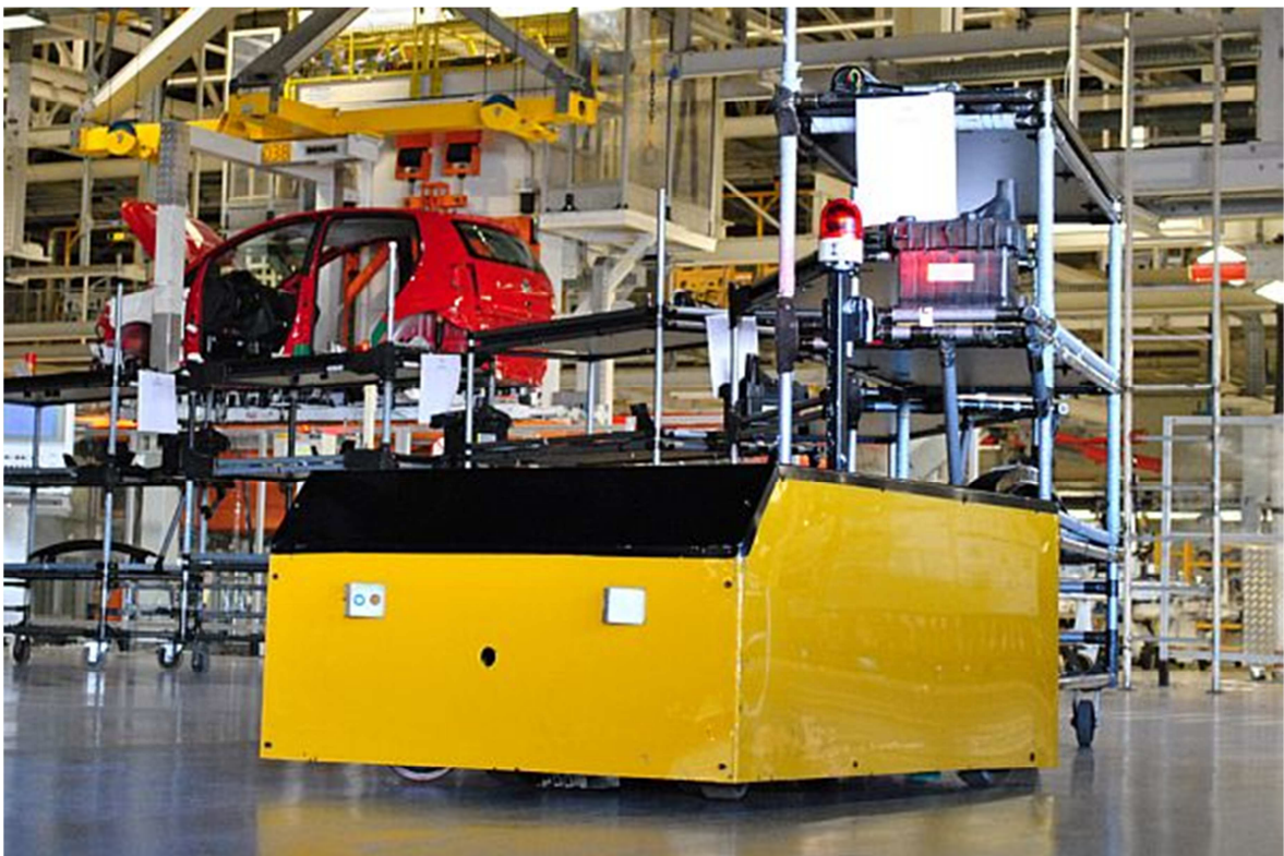
Figura 2 - Exemplo de AGV ( Automatic Guided Vehicles )
