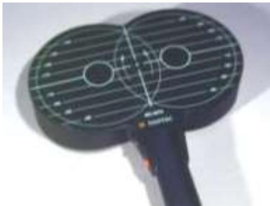
**Figura 12 – (b) Bobina coplanar, oito**
