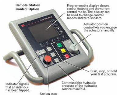
*Figura 42 Remote Station Controller (RSC)*
