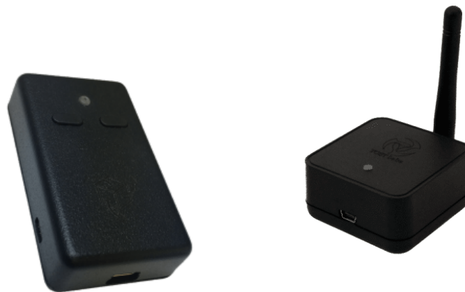
Figure 3.2: The IMU wireless sensor and a wireless dongle (receiver) 3-Space Sensor , from Yost Labs .
