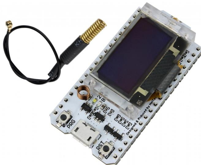
Figura 6 – Microcontrolador WiFi LoRa 32.(HELTEC, 2018)
