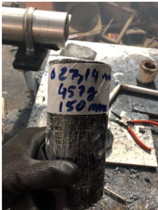
Figure 5 – Cataloged fuel grain after production.
