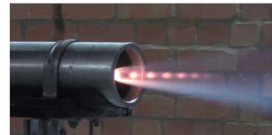
Figure 4 – Diamond shockwaves and smoke in exhaust of the motor.
