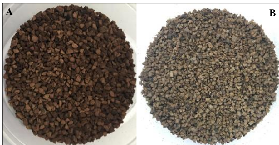
Figura 11 – Hydrochar: (A) HT (hydrochar de Tingui) e (B) HTK (hydrochar de Tingui com K_2CO_3 ).
