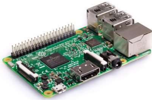
Figura 9: Raspberry Pi 3 Model B [10]
