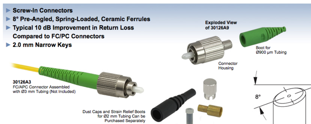
Figura 15 – Conector FC/APC. [33]
