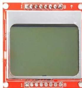
Figura 8 – Display LCD 5110 Vista Frontal (FLIPFLOP, 2016).
