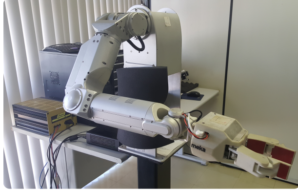
Figure 4.2: Meka robot available at LARA at UnB (A2 Arm from Meka Robotics)
