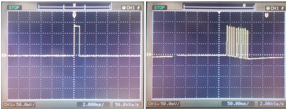
Figure 3.6: Voltage output measured from board with 1 and 10 pulses.
