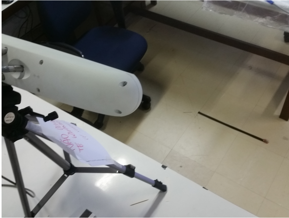
Figure 3.4: Arrangement used for the experiments. Polaris Spectra is positioned facing the floor, where a line indicates the desired path, namely, the reference path.
