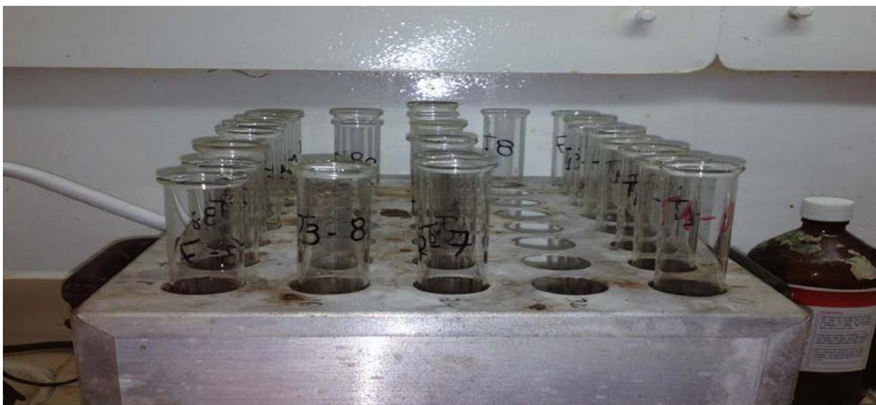
Figura 9: Tubos no bloco digestor.
